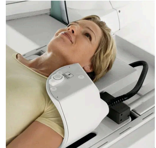
A shoulder coil for MRI. Coil geometry needs to be compliant with many factors, including the sample! Solenoids are often not possible.
