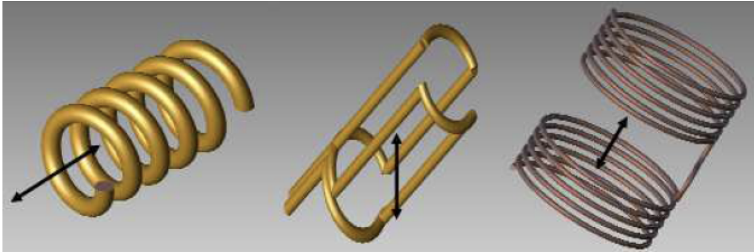
A solenoid coil (left), a saddle coil (middle) and a Helmholtz coil (right). The three of them yield a homogeneous magnetic field in the center with a direction represented by an arrow. (from A.J. Perez-Linde, PhD thesis, Nottingham)
